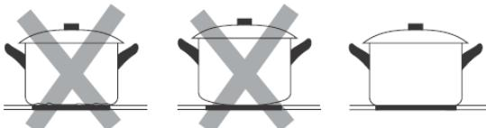
Make sure that the base of your pan is smooth, sits flat against the glass, and is the same size as the cooking zone. Use pans whose diameter is as large as the graphic of the zone selected. Using a pot a slightly wider energy will be used at its maximum efficiency. If you use smaller pot efficiency could be less than expected. Pot less than 140 mm could be undetected by the hob. Always centre your pan on the cooking zone.
