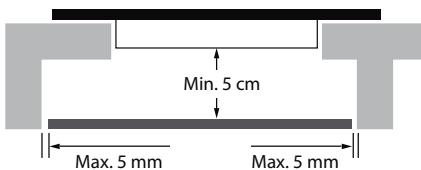
There are ventilation holes around outside of the hob. YOU MUST ensure these holes are not blocked by the worktop when you put the hob into position.
